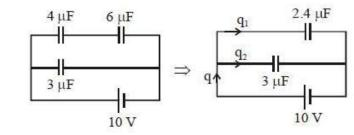
So total charge flow =  $q = 5.4 \mu F \times 10V$ = 54  $\mu F$
