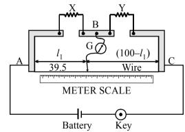
In a meter bridge, as shown in the figure, it is given that resistance  $Y = 12.5 \Omega$  and that the balance is obtained at a distance 39.5 cm from end A (by Jockey J). After interchanging the resistances X and Y, a new balance point is found at a distance  $l_2$  from end A. What are the values of X and  $l_2$ ? (1) 19.15  $\Omega$  and 60.5 cm (2) 8.16  $\Omega$  and 60.5 cm (3) 8.16  $\Omega$  and 39.5 cm (4) 19.15  $\Omega$  and 39.5 cm
